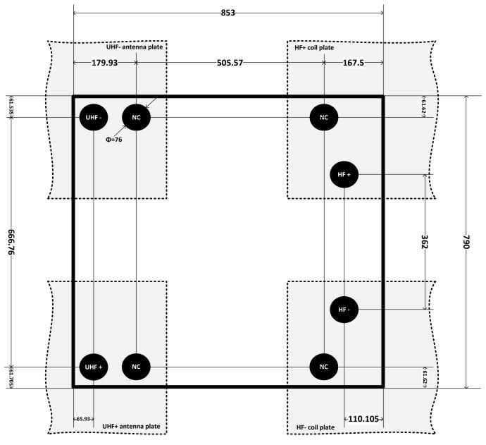
The chip size is calculated including the scribe line. UHF antenna plates and HF coil plates are added here only to illustrate inlay assembly option.
